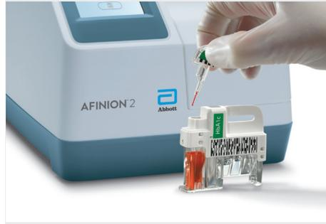
**3** Place the test cartridge in the analyzer and close the lid. The processing starts automatically.
