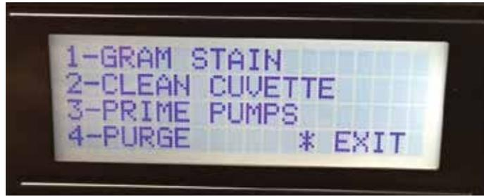
**NOTE:** The Gram Stain command will fail to start if the instrument is due for a required Bleach or Scrub cleaning cycle.
