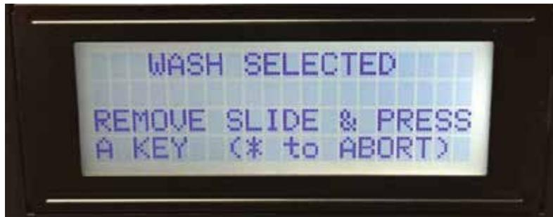
9.1.4 Press **any key** on the key pad to run the Wash Cycle
