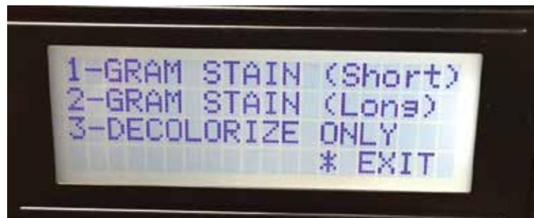
There are two sets of pre-programmed stain delay times, a short or a long option. The soak times for crystal violet, Gram's iodine, and safranin are determined by this selection. Note that the three soak times (for CV, GI and SAF) of each of the three sets may be altered as desired by the facility administrator. The default settings are:
